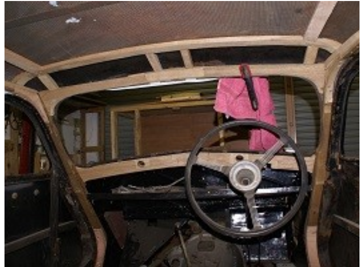
Above front timbers of George and below the 'A' pillar fitted
