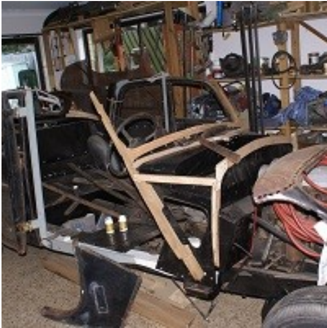
Above front timbers of George and below the 'A' pillar fitted
