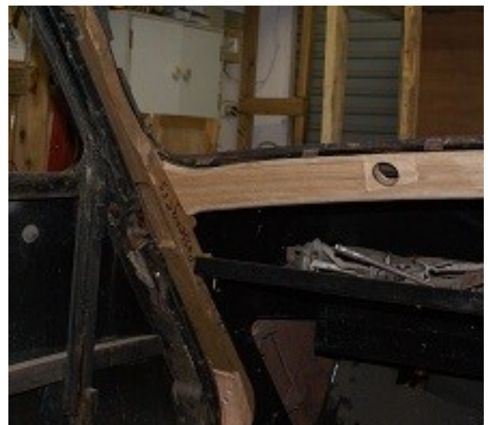
Above front timbers of George and below the 'A' pillar fitted
