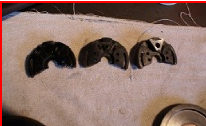
Above: Three Bakelite trafficator bases broken in the same place
