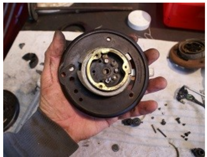
Above: Long bolts secured and the brass ring fitted
