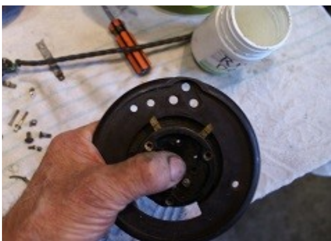
Above: Long bolts secured and the brass ring fitted
