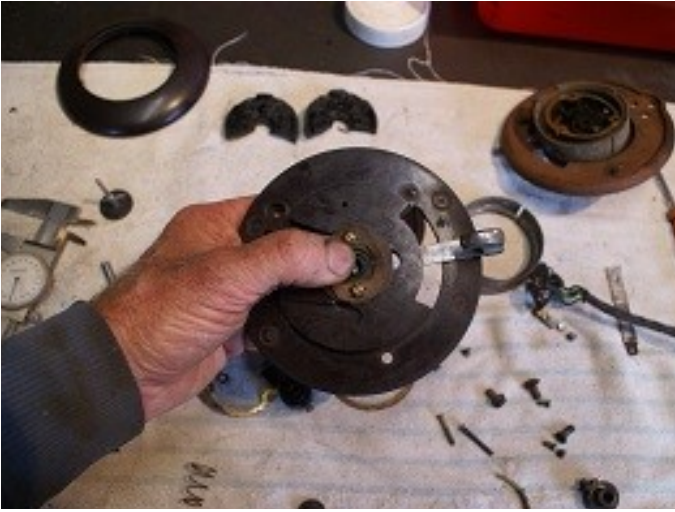
Above: the horn push contacts being fitted
