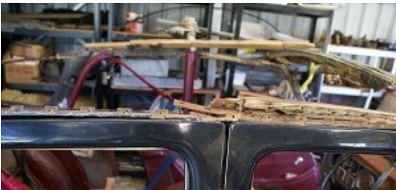
Above: The cant rail smashed
