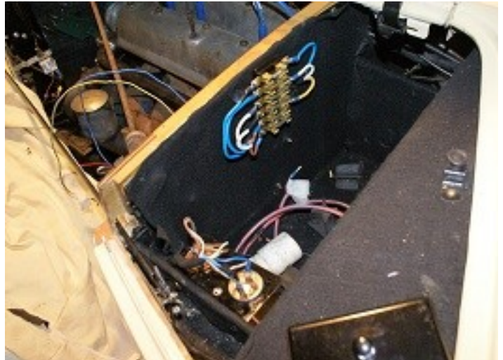
Above: Fuse box and flasher units
