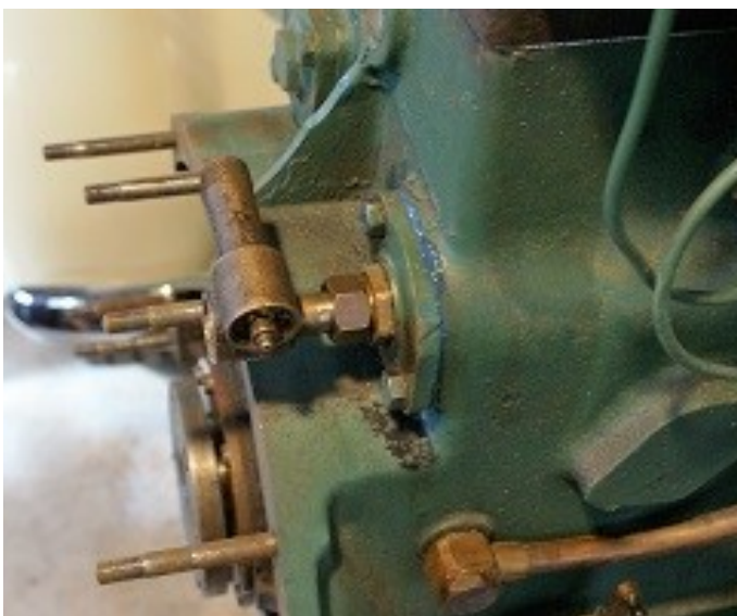
Below Tacho drive fitted to inlet cam
