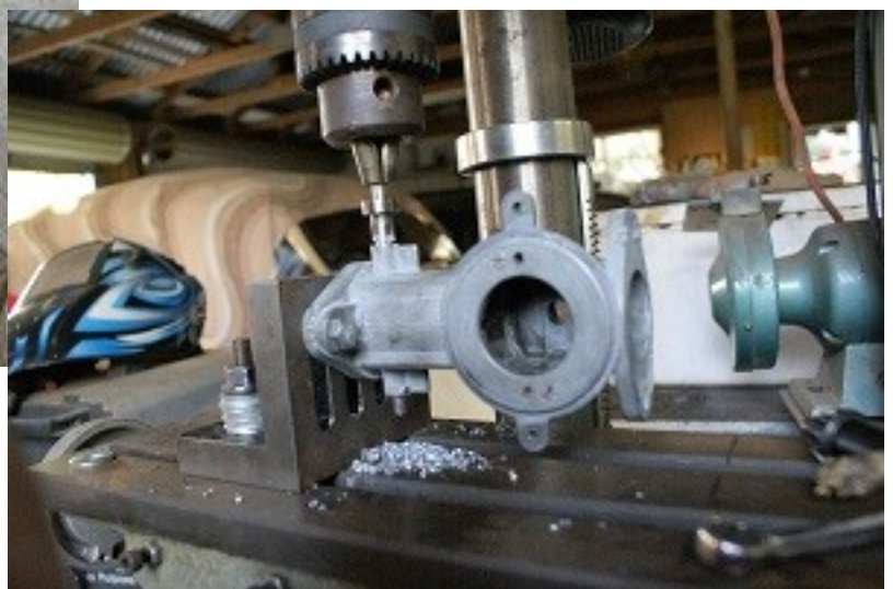
Above: The butterfly shaft being reamed
