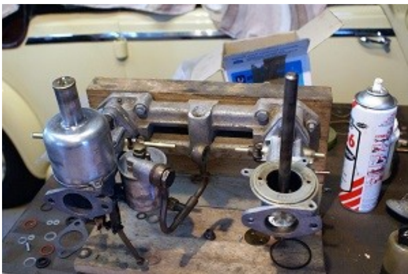
Above: The carburettors being assembled
