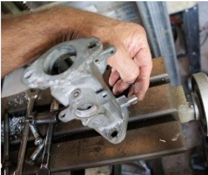
Above: Butterfly shaft bushes being pressed into position
