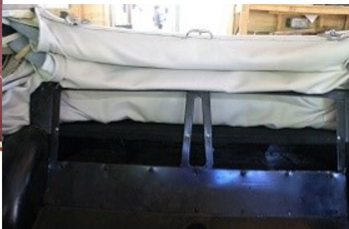
Above: Rear window has fallen into the hood box
