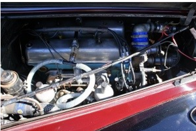
Above: The thermostat located in the top hose
