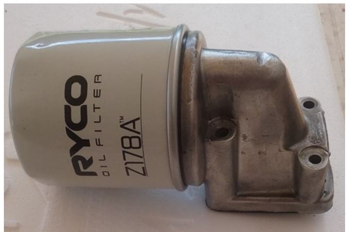
Oil filter as fitted to previous engine. New assembly takes a Repco Z178A
