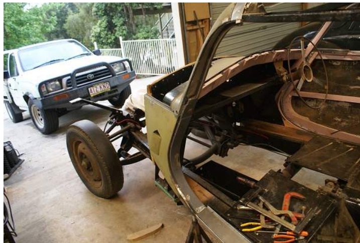
Steel skin for the door post and the square shape to sit against the quarter window
