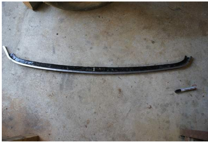
Water exclusion channel welded to header stick steel skin
