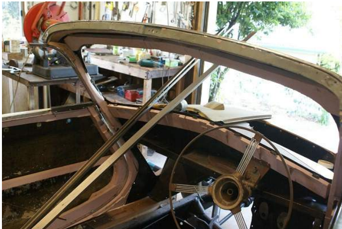
Header stick and steel skin fitted
