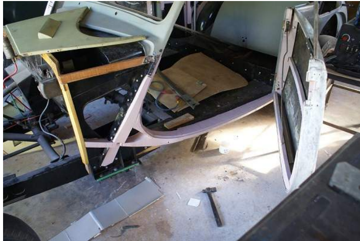
Quarter panel and outer sill timbers fitted
