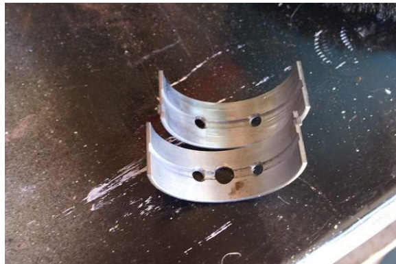
The Nissan bearing with its new oil hole and the chamfered edge on the original oil holes with central groove.
