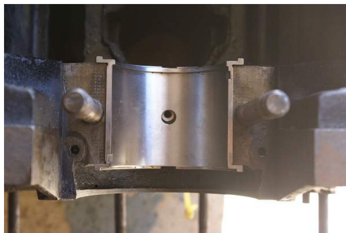
Bearing housing over the oil port
