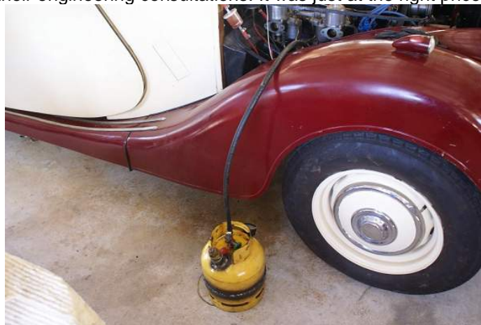
Oiling vessel attached to the filter inlet.
