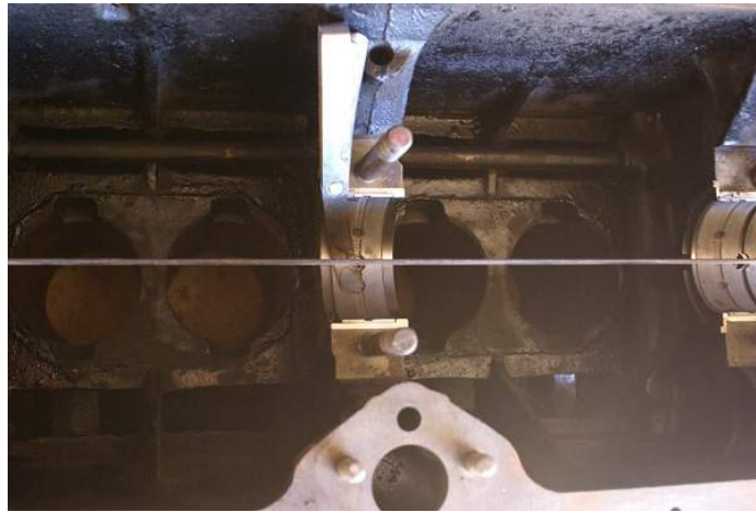
Straight edge over the bearings
