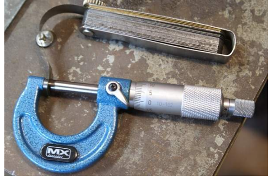
Gear end float checked against a micrometre
