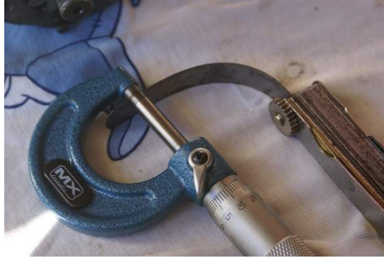
Gear gap against pump body checked
