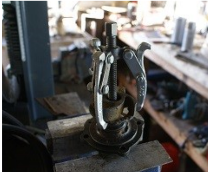
Above: A small workshop puller being employed to take the impeller off
