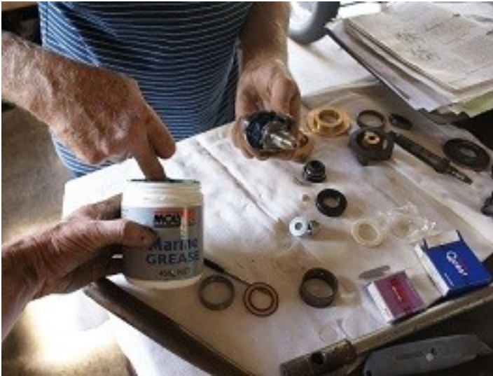
Above: The parts laid out and the application of marine grease and below: refitting the shaft and bearings
