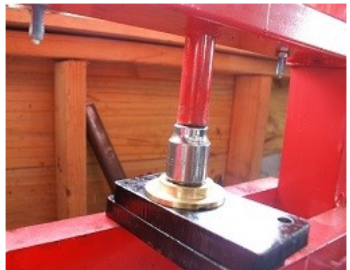
Above: the outer flange tapped into place
