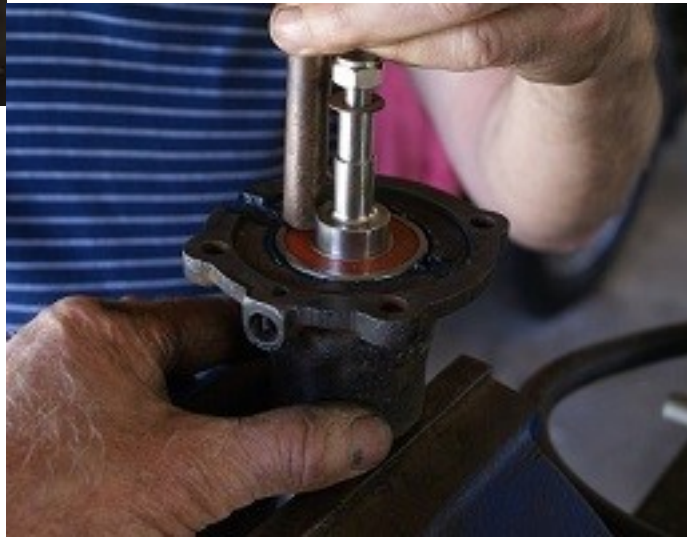
Above: the bearing being tapped into place
