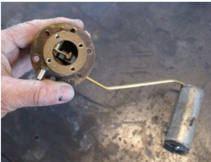
Above: The sender unit with completed mechanism and float
