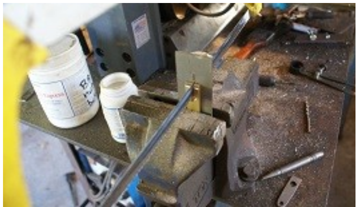
Above: Hacksaw guide and the clamping bolt in position
