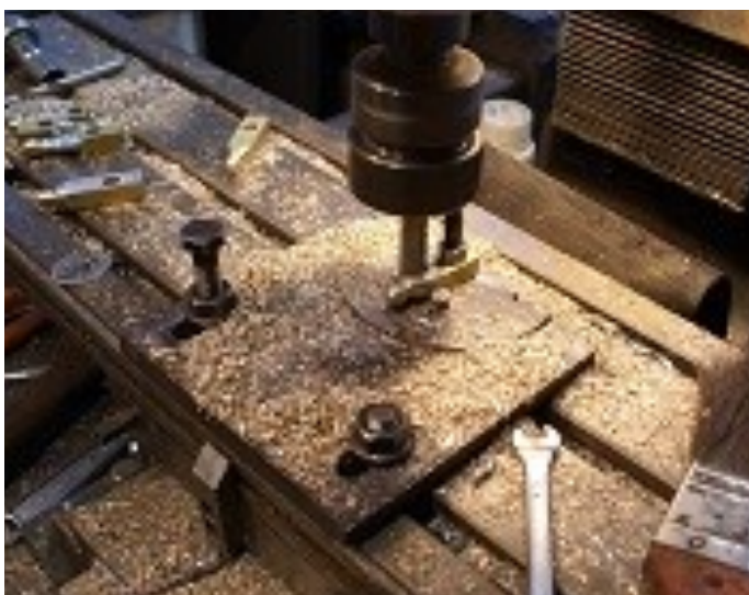
Above: Milling the magneto control arm and
