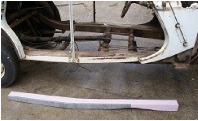
Above: The sills ready to be fitted
