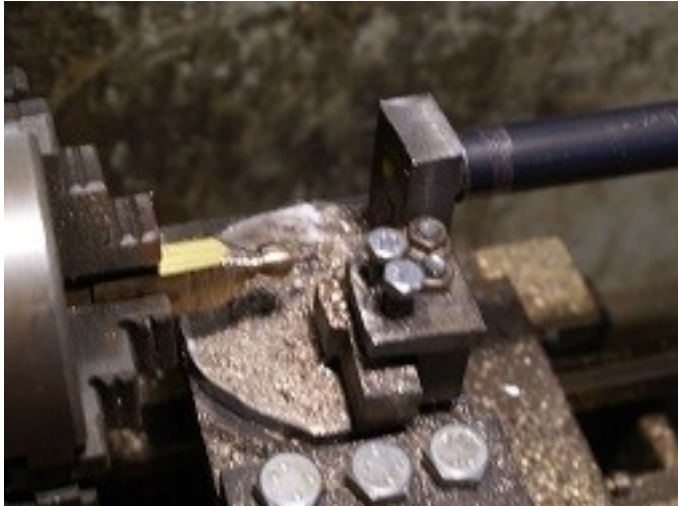
Above: Ball being cut into the magneto control arm
