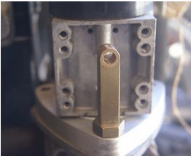
Above: The magneto with the drilled and tapped holes.
