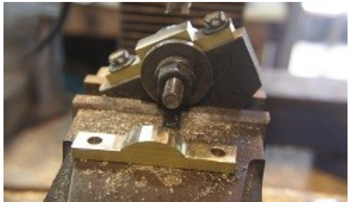
Above: The magneto attachment with hole template above it and below: the milled and drilled bar
