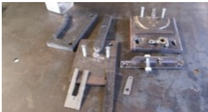
Above: The jigs and templates used to make the magneto advance and retard mechanism for Edward, the 1929 Riley Roadster.
