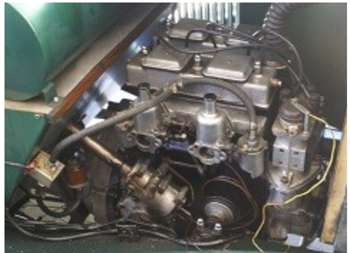
Above : Riley 9 with twin SU carbies and the BTH (British Thomas and Houston magneto). You might recognise it as the one in Mathew Schooneveldt's Riley
