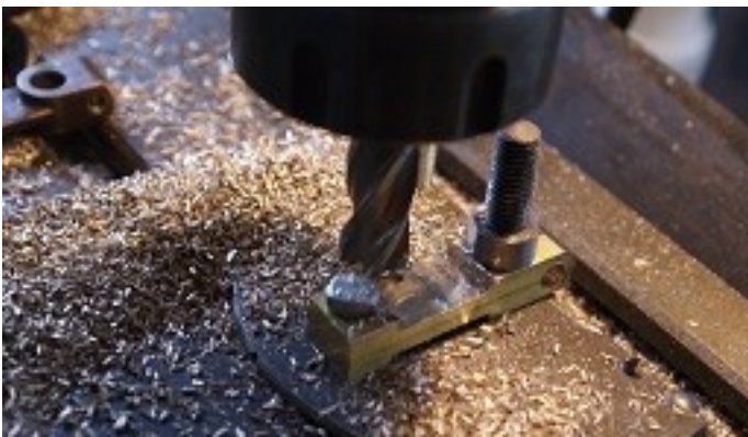
Above: Milled and drilled control arm and below: The control arm sides milled
