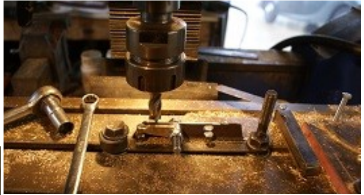
below: Milling the sides of the magneto control arm
