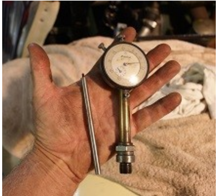
Above: A fairly old dial gauge fitted into a copper tube and over an old spark plug with an extension to reach the piston.
