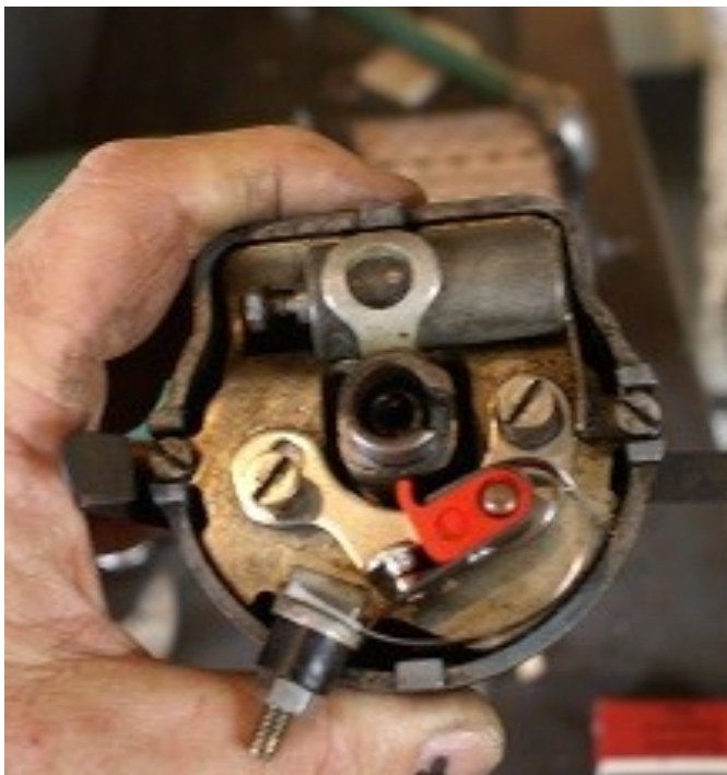
Above: The L10 points fitted into a spare distributor but without adjustment to create a gap between the points
