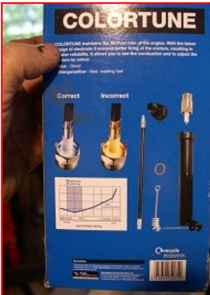
Above: The Colortune assembly fitted to number one combustion chamber. The mirror is at the top of the column. Below: The Colortune guide
