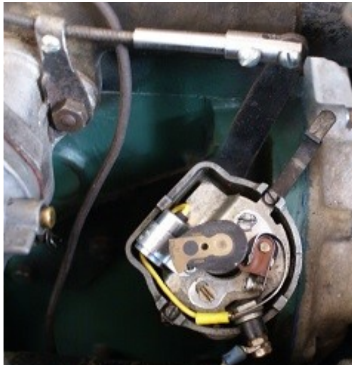
Above: Mechanical advance with the distributor in place
