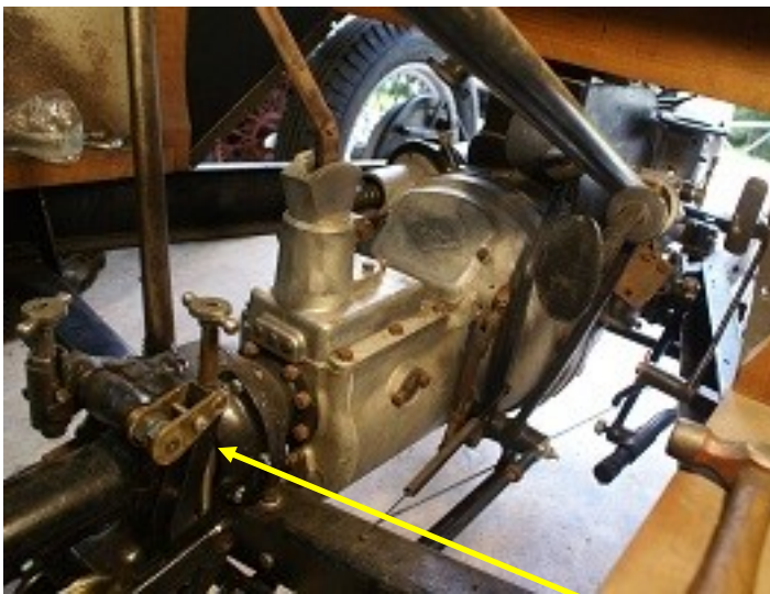
Above: the footbrake mechanism with fixing bracket
