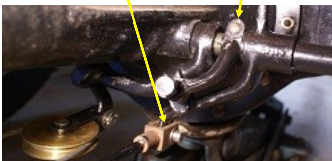
Below: brake rod clevis pin and bicycle bolt in place
