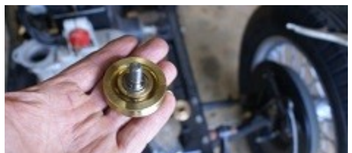
Below: Queensland made pulleys with needle bearings on a stainless steel stud
