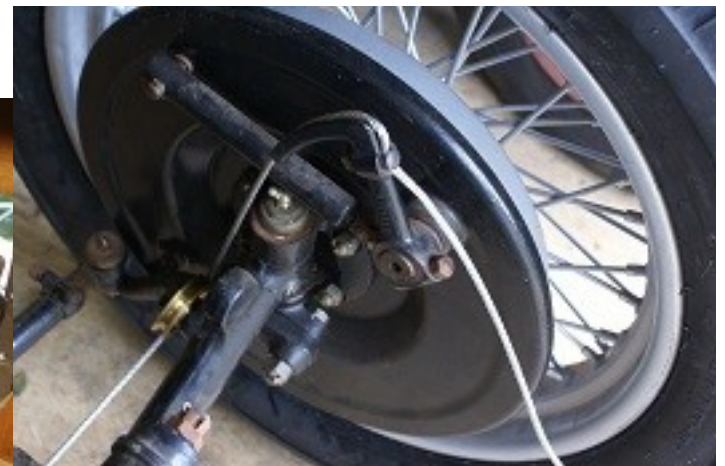
Above: brake cable fitted to front left wheel brake mechanism and below the cable threaded around the braking pulleys
