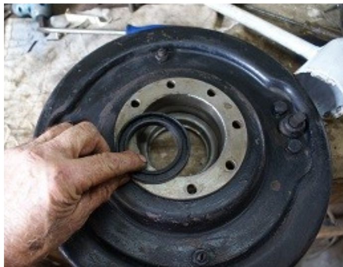
Above: The diff seal being fitted
