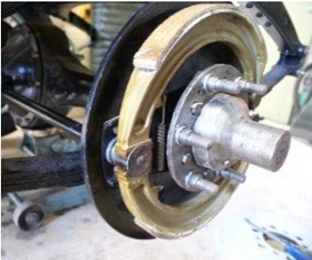
Above: The hub, brake shoes and brake rod and below: brake shoes in profile
