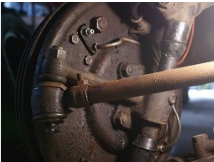
Above: The flaring tool with the button and under the tool you can see the new joiner
