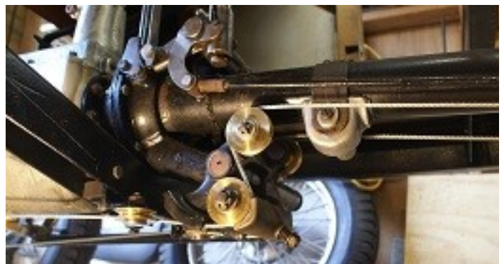
Above: the footbrake mechanism with fixing bracket
