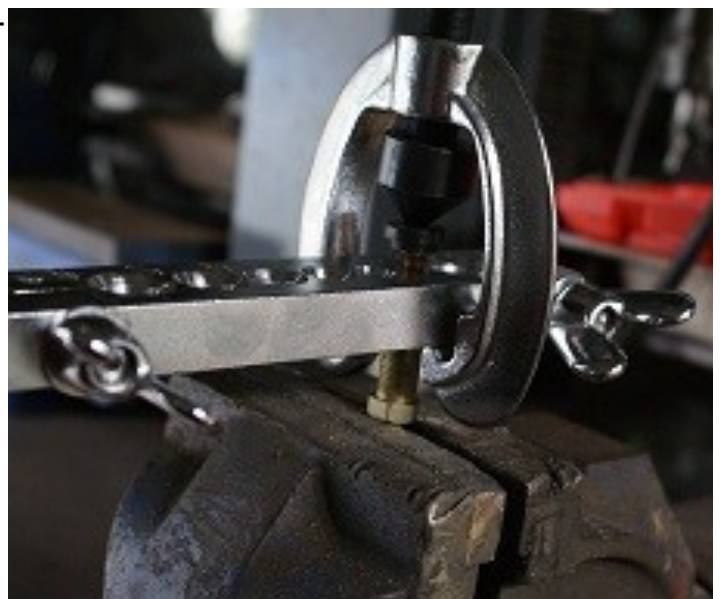
Above: The flaring tool with the button and under the tool you can see the new joiner
