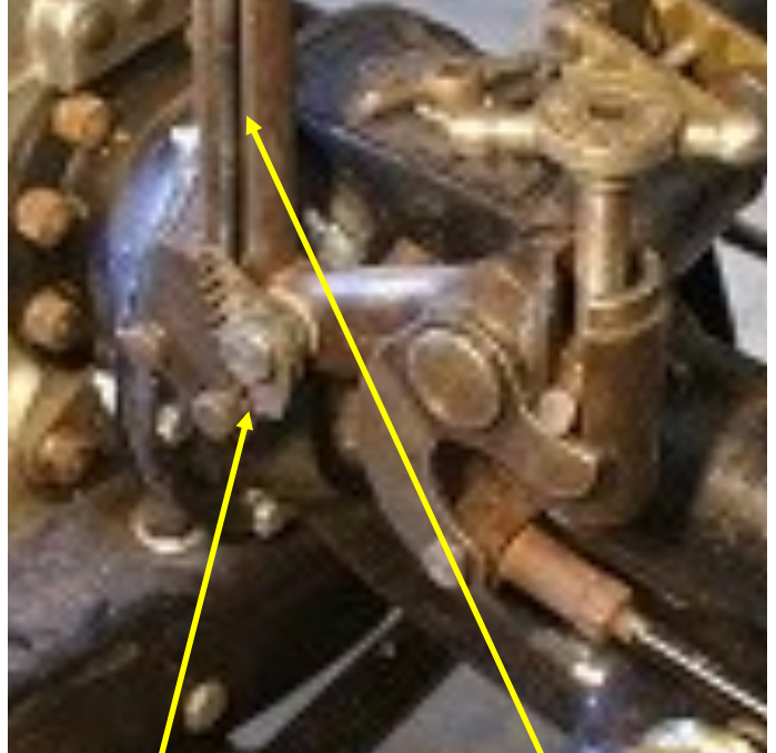
Above: The ratchet pin and the actuating rod
