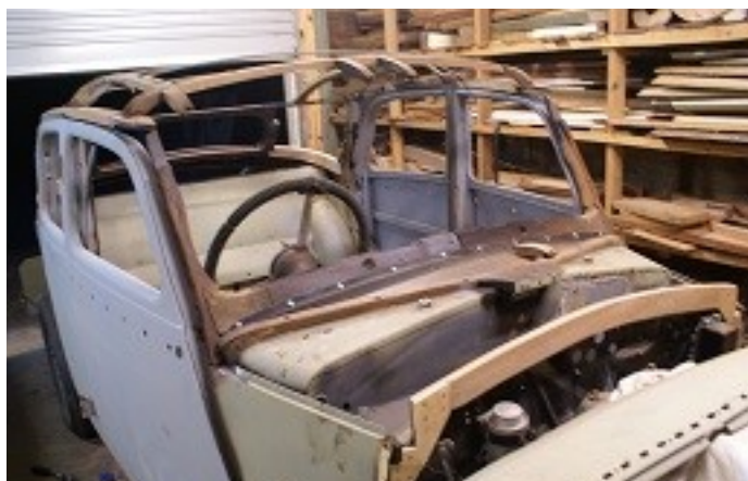
Above: Aaron Butterfield's RMB undergoing a reframe.
