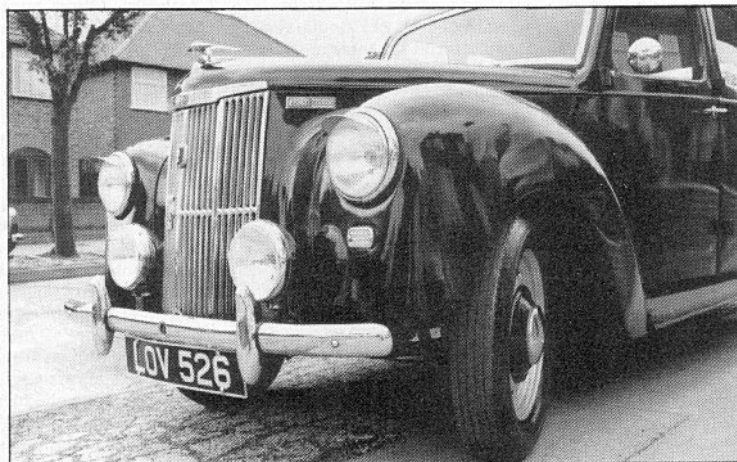
Most owners fitted spotlights to their Ford Prefects because the standard headlamps were next to useless.
