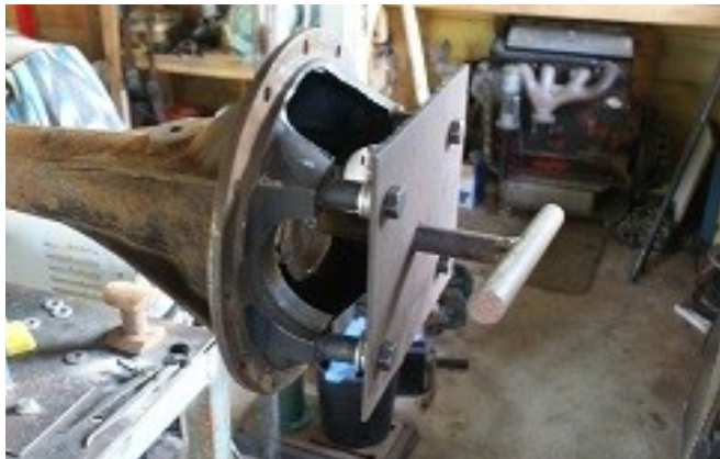
Above: Diff with pinion extractor
