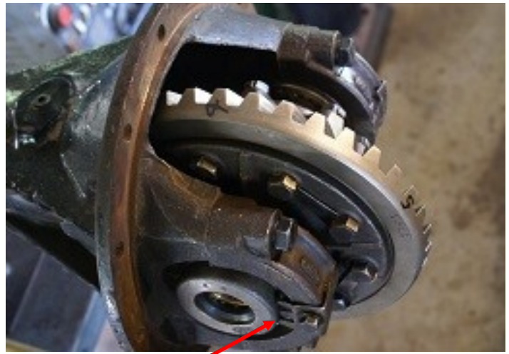
Below: crown wheel fitted
