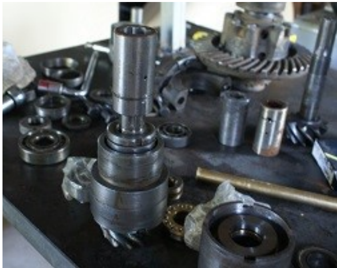
Above: The pinion reassembled with the muff coupling
