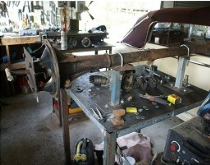
Above: Diff rebuild cradle
