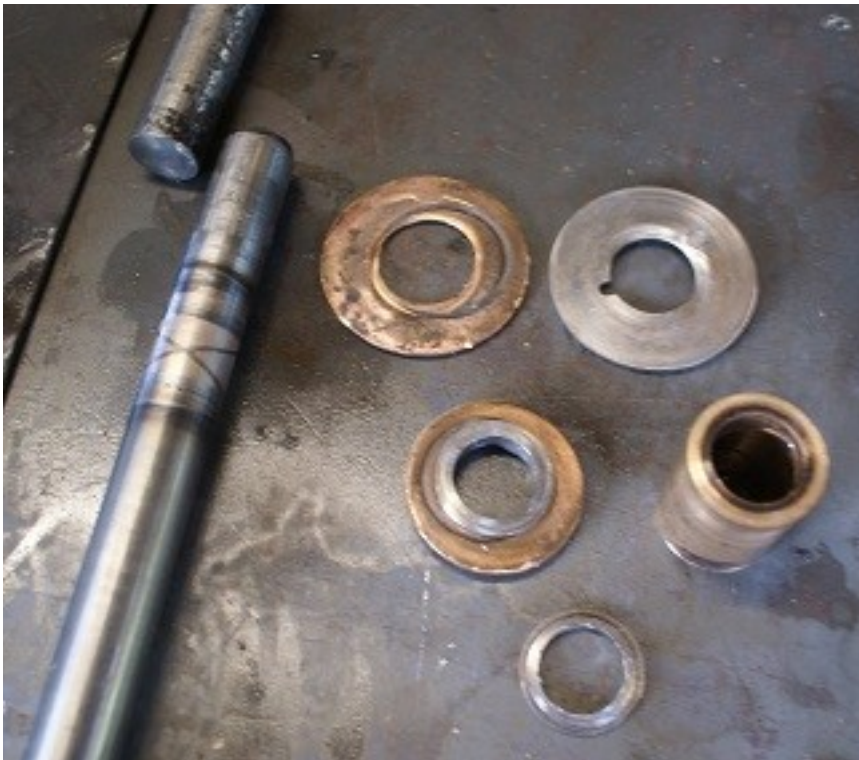
Above: From the left the lay shaft with its peculiar marks, the brass component of the front lay shaft thrust washer and next to it the steel part and at the bottom of the picture the centre piece that had embedded itself into the gearbox.
