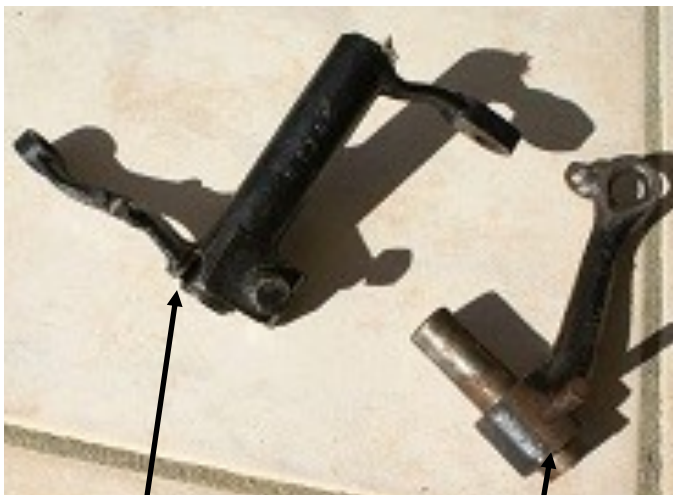
Above: Busted clutch operating lever and busted clutch compensating lever
