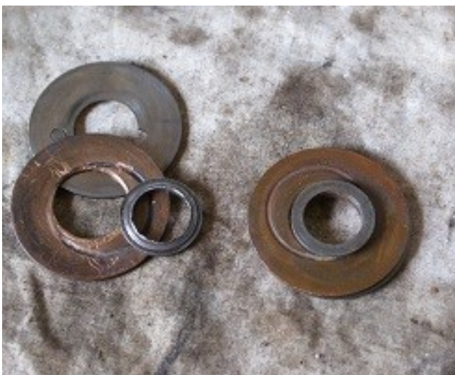
Above: The broken thrust washer on the left compared with the washer obtained from spare parts
