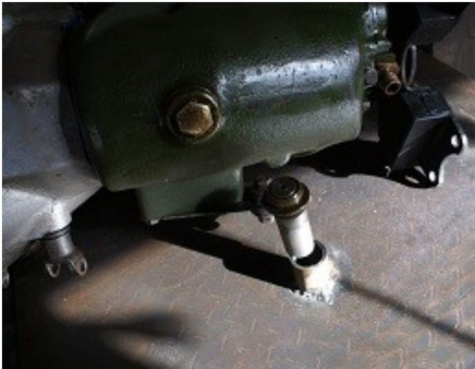
Above: swivel post, socket and drain plug
