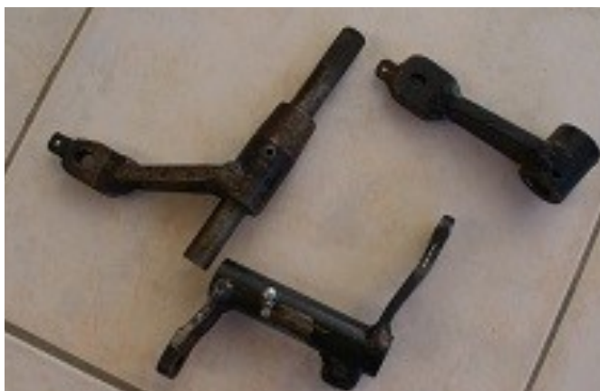
Above: Busted clutch operating lever and busted clutch compensating lever
