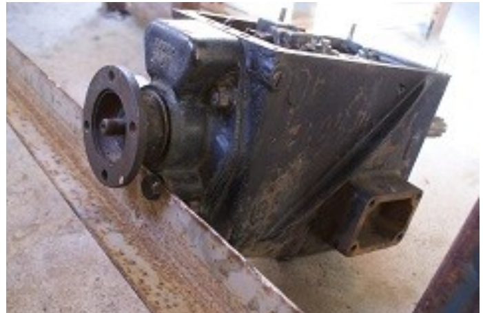
Above: The gearbox bolted to the angle iron giving it stability while the castellated nut was released from the flange.
