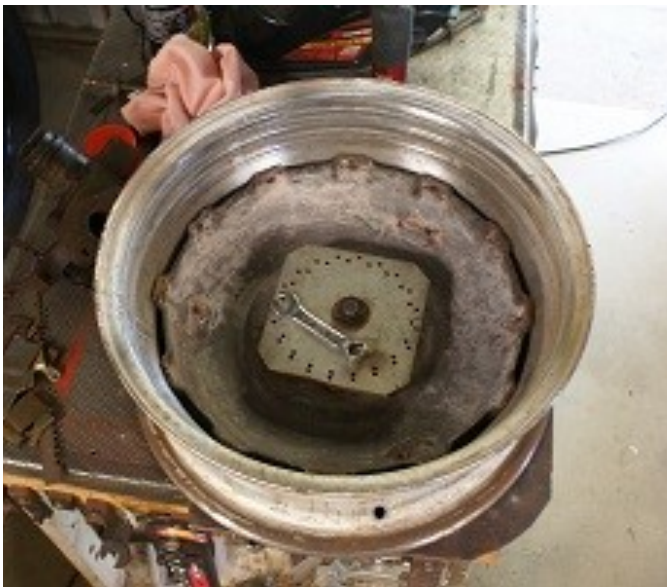
Above: Jig for welding Modern outers to Riley inner rims.
