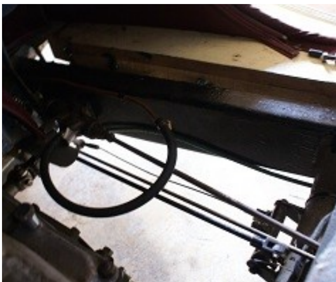
Above: Master Cylinder assembled and fitted to linkages
