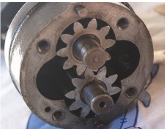
Above: worn oil pump gears
