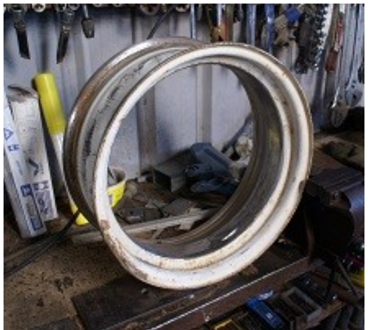
Above: Nissan Navara outer rim separated from inner rim
