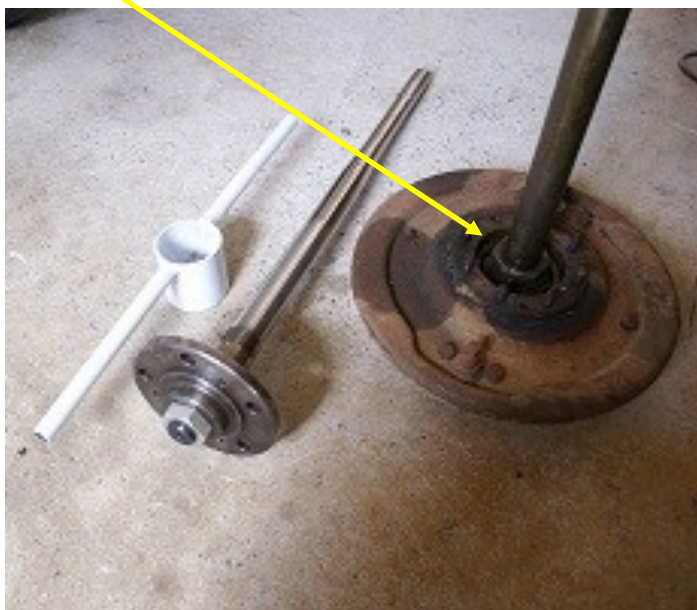
Below: The old half shaft on the hub with the nut, a new half shaft, and tube spanner
