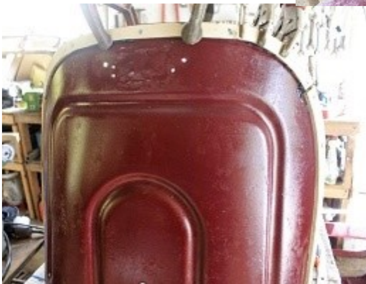
Above: Marine five-ply strips bolted and glued to seat backs
