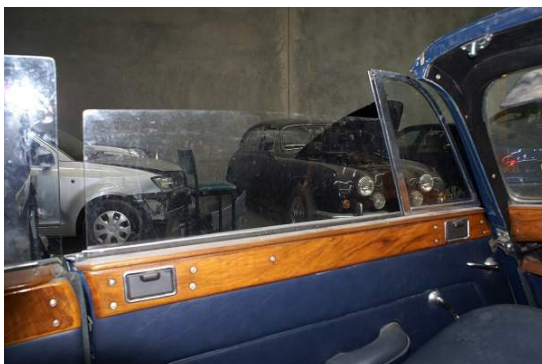
Picture of a quarter window and winding window track.
