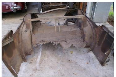
that it was unusable and so the electrical components were removed and the scuttle went onto the ute for disposal. The tub section was in similar condition so it was cut through along the sides of the boot leaving the mudguards and sides of the car for later use and the centre of the tub also went onto the ute. The reader may lament the careless discarding of Riley parts but in my defence, I have not yet met a person who could restore humpty dumpty after this kind of fall.
