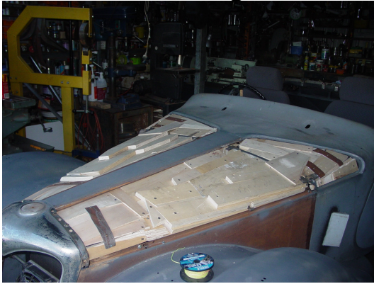
Engine space blocked out.
