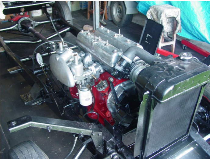
Note the oil filter adaptor.
