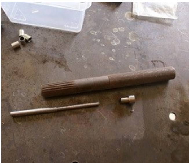
Above: The 2 BA fixing bolt allows me to fit another cutter when required
