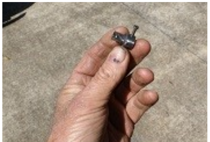
Above: The 2 BA fixing bolt allows me to fit another cutter when required
