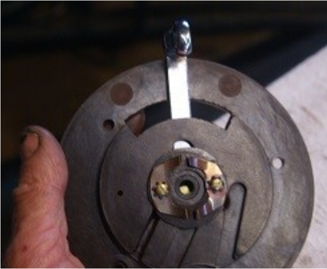
Above: The horn contacts with their bolts at 3 and 6 O'clock and below when the horn contact is removed the trafficator arm retaining bolt is revealed.
