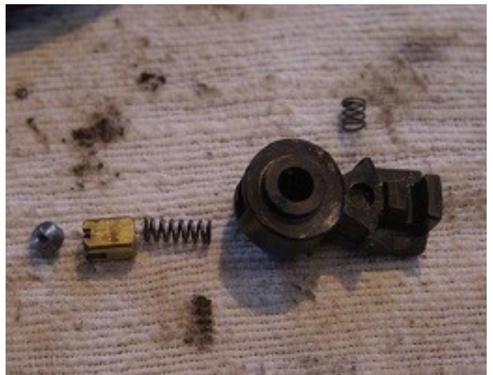
Below: Trafficator Bakelite centre with spring, carrier, and wheel
