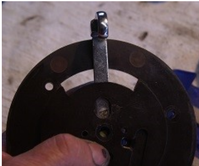
Above: The horn contacts with their bolts at 3 and 6 O'clock and below when the horn contact is removed the trafficator arm retaining bolt is revealed.
