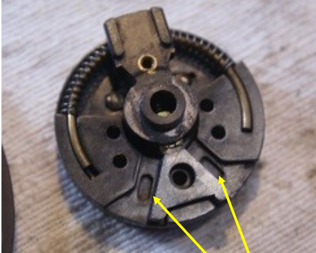
Above: The centre piece with trafficator selector, the springs and the triangular pivot
