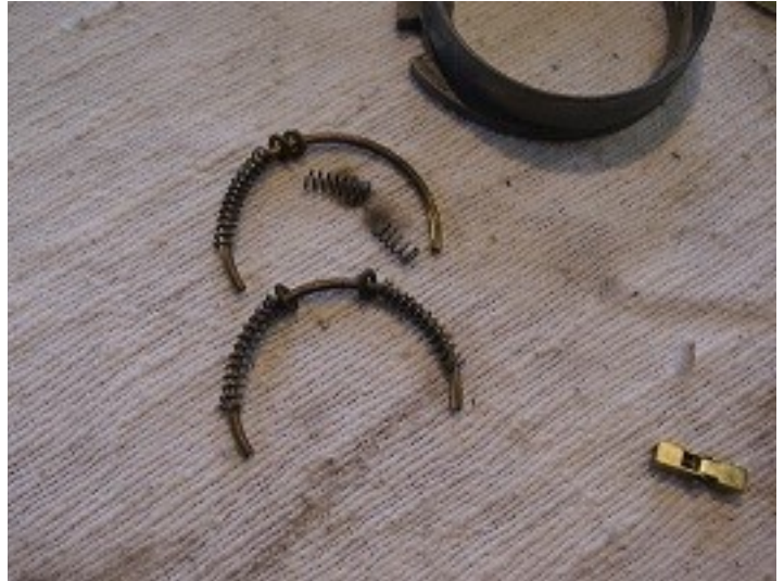
Above: The broken return spring
