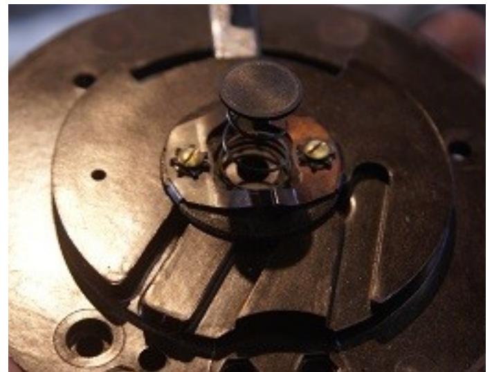
Above: The horn push contact with its spring and button. The spring and button the other way up.
