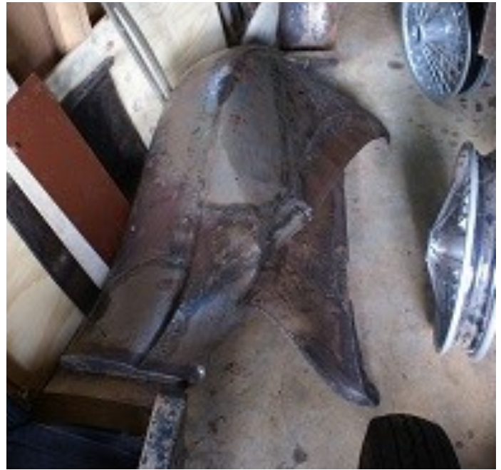
Above: A remarkable amount of welding and panel work has produced a marvellous result. Notice the patches.
