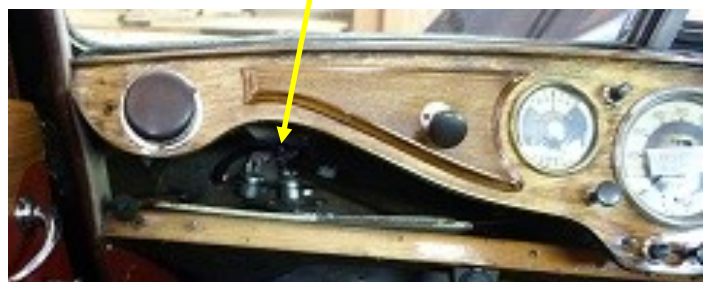
Below: Flasher units fitted under the dash
