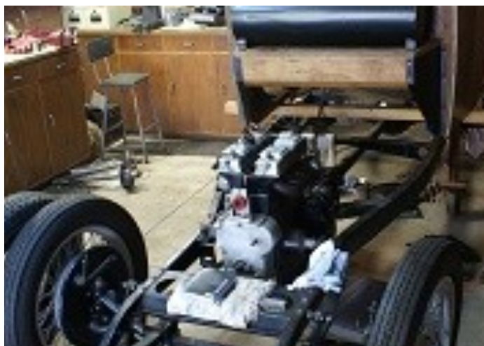
Above: Another photo of Edward in Jane's garage. The engine is installed but electrical items and carburettors are in boxes.
