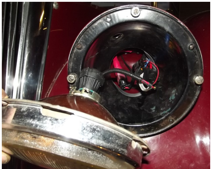
Above: Headlight fitting into a pod that has been cut out to accommodate the bulb rear projection and below: Ballast and controller in headlamp flaring and control unit mounted in the engine bay
