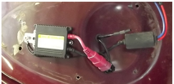
Above: Headlight fitting into a pod that has been cut out to accommodate the bulb rear projection and below: Ballast and controller in headlamp flaring and control unit mounted in the engine bay
