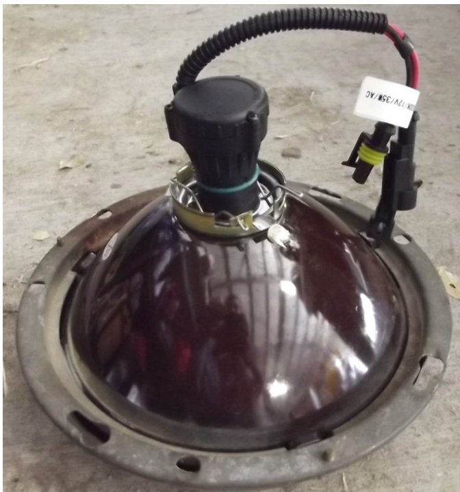
Above: Bulb mounted in reflector. Note the large rear projection of the electro mechanical dipper
