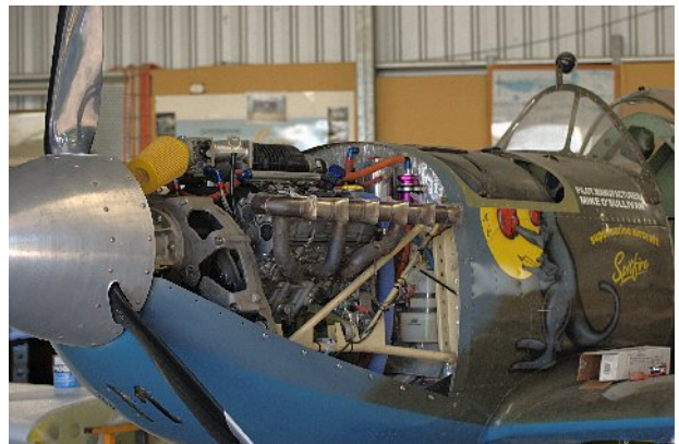
Honda-built GM Isuzu V6 in position.
