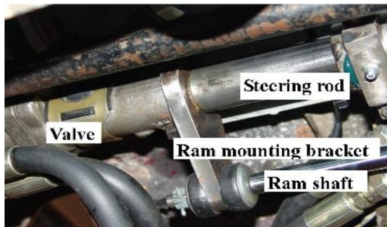
Photo from rear showing ram mounting bracket and control valve screwed onto the new steering rod as described in C.
